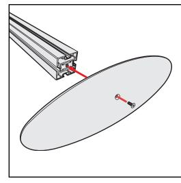
Base Plate & Extrusion Connection
